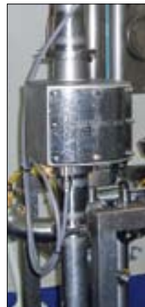
MoistScan MA700 in an Australasian processed cheese factory controlling steam injection cookers for quality and yield maximization.
