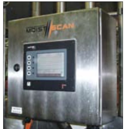
MoistScan MA700 in an Australasian processed cheese factory controlling steam injection cookers for quality and yield maximization.
